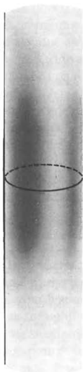
FIGURE A.14 Gaussian curvature of a cylinder is zero.
