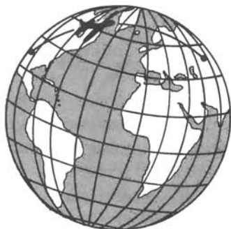
FIGURE 2.1 The shortest path between two points on a sphere is an arc of a great circle (a circle whose center is the center of the sphere and whose radius is the radius of the sphere, e.g., the equator).
